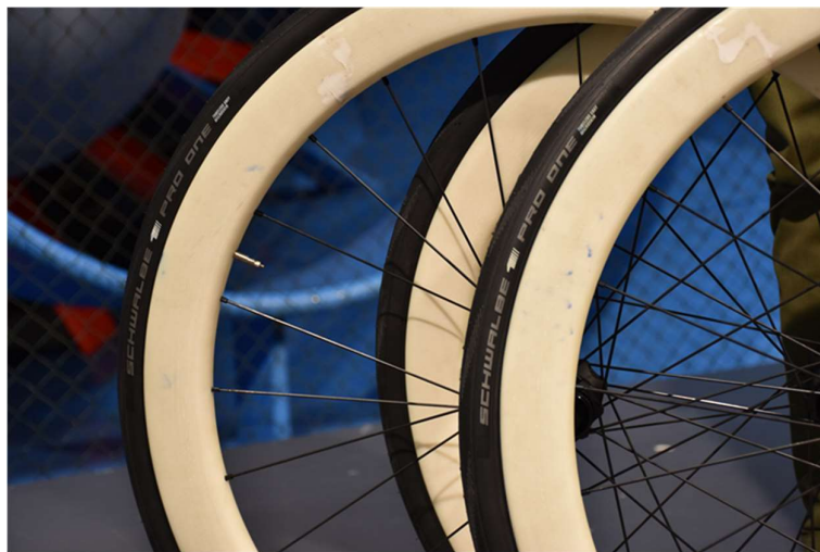
Figure 5 Photograph of the 3D printed ABS prototypes
